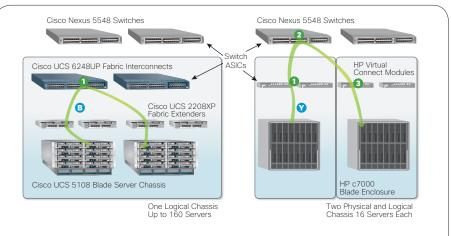
Figure 2. Cisco UCS and HP BladeSystem Traffic Flow To and From a Blade in Different Chassis
