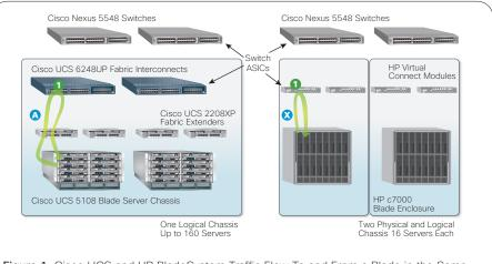
Figure 1. Cisco UCS and HP BladeSystem Traffic Flow To and From a Blade in the Same Chassis
